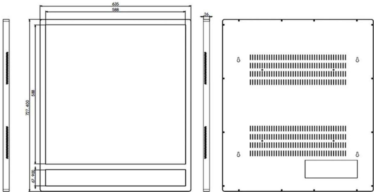
This machine is designed to display two 35.7 inch screens. The total width of the machine is 635mm, and the total height is 717.4mm. The inner screen width is 588mm, and the inner screen height is 588mm. The bottom bezel has a height of 67.9mm. The machine has a depth of 26mm. The back view shows two rows of ventilation holes and four mounting points.
