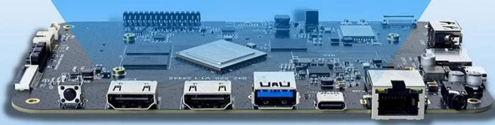
Rockchip RK3588 ARM (Cortex-A76 Cortex-A55) Mali-G610 NPU 6 TOPs LP. \*LCD: MIPI EDP. \*I2C. \*TF PCIE. \*UART GPIO. 12
