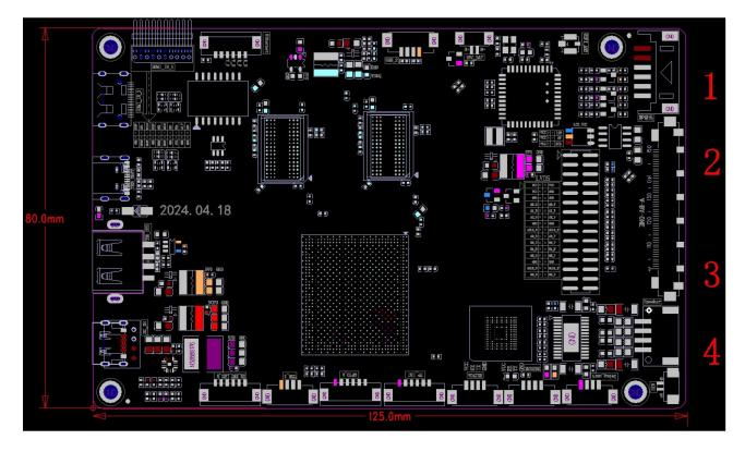
PCB: 4-Layer Board Size: 80mm\*125mm, Plate thickness 1.2mm Screw hole specifications: Φ3.0mm x 4
